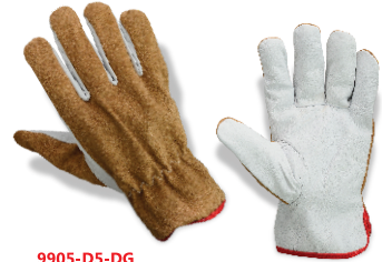
9905-D5-DG Premium quality Goat skin leather Keystone thumb Brown split cowhide leather back Zigzag stitched elastic on wrist Cotton hemmed Size 10 inch
